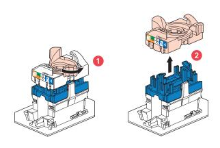
This system allows you to spread pairs before fitting them onto the connector.
