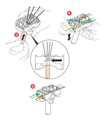
Spreading the cables ensures that a pair-breakage distance of 13 mm is kept between each pair.
